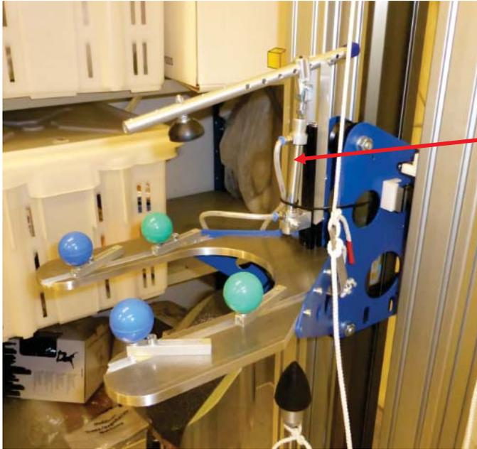
Pneumatic cylinder aimed to clam the helmet during the vertical drop.
