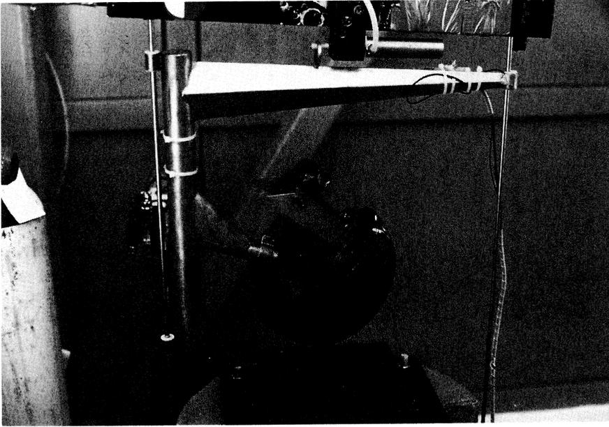
FIGURE 14.7. Typical helmet-impact vertical-drop test setup.
